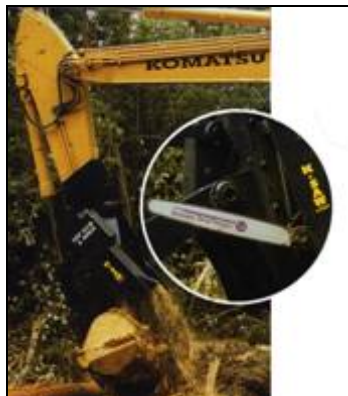
Figure 1 The K-saw commonly attached to a hydraulic excavator.
