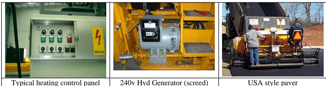
**Figure 1** Paver high voltage electrical systems.
