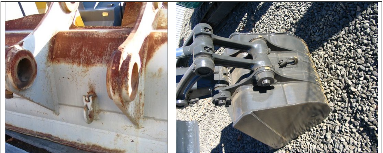
Figure 1 Typical lugs welded to the external side of the bucket.
