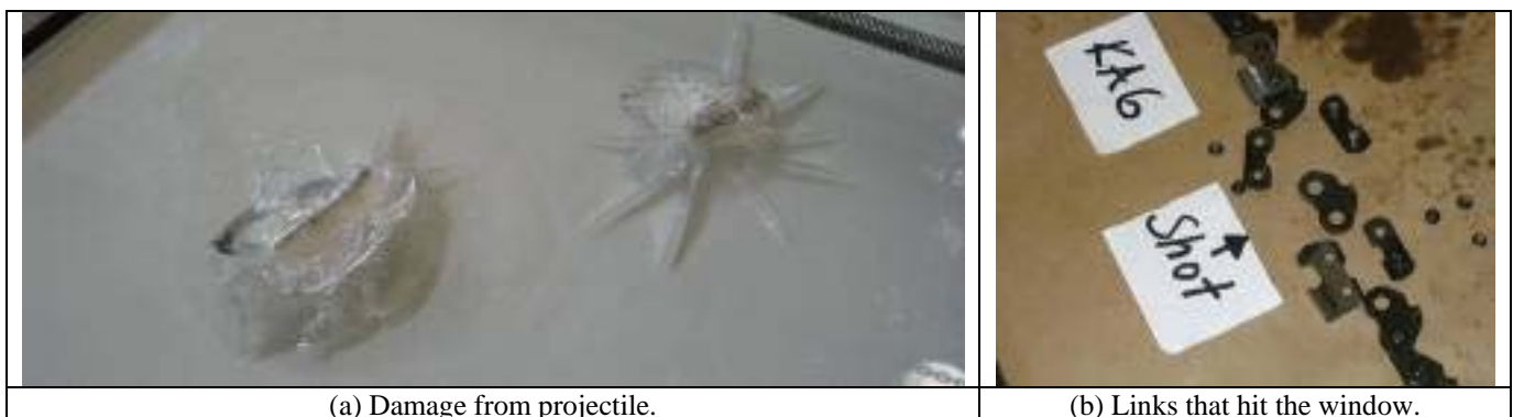
Figure 4 Photos from type 2 test (refer to Tables 2 and 3 for more details).
