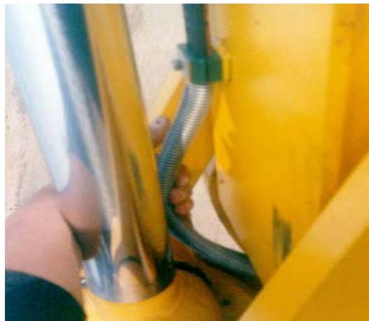
**Figure 9 – Checking Hose Clearance**
