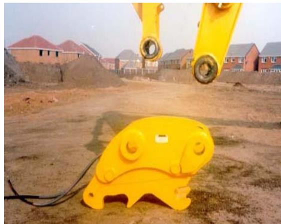
**Figure 8 - Positioning the Quick Hitch**
