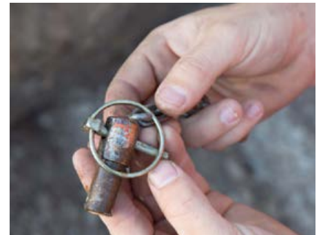
Photo 4: Shows the safety pin and lynch pin from photo 3.
